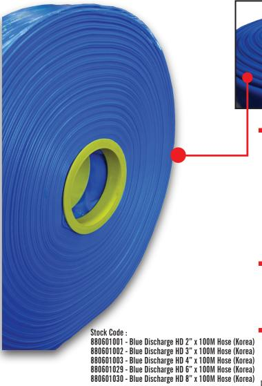
Polyurethane Blue Discharge lay-flat Hose that resists kinking and twisting. It is designed as a standard duty hose for water discharge in industrial and construction applications, is strong and economical, and rolls up flat for easy storage. Reinforcement includes spiral plies and longitudinal synthetic cords for excellent burst resistance. It resists abrasion and tears, and is usable at higher pressure. Other varieties for higher pressures alternate materials are also available.
