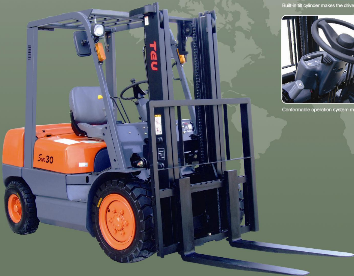
Built-in tilt cylinder makes the driver cab more spacious
