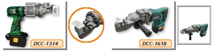
The DCC-1618 is a cordless cutter with head that rotate through 345 for use in truly awkward locations. Handling rebars of up to 16mm and 13mm 490N/mm<sup>2</sup> tensile strength respectively, they are equally suitable for mesh and bolts and, since they do not produce sparks or generate heat, they are particularly effective in rescue operations. The 4.5kg DCC-1314 is the smallest brother of DCC-1618.
