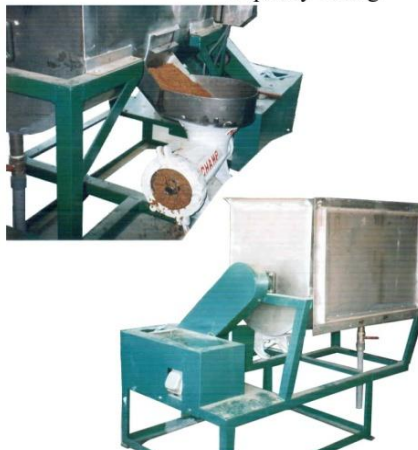
Pelletized Machine 5HP/3PH c/w gear box with #52 Meat Mincer Capacity : 30kg
