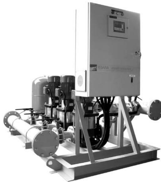
The EBARA Hydro Booster system consists of two or more EVM pumps coupled in parallel and mounted on a common baseplate, integrally provided with a EBARA Hydro Controller electrical cabinet and all the necessary common pipe work and fittings. All EBARA Hydro Booster system is factory assembled and tested, pre-set according to customer requirement. It is ready-to-connect at site. Scope of supply includes instruction manual.
