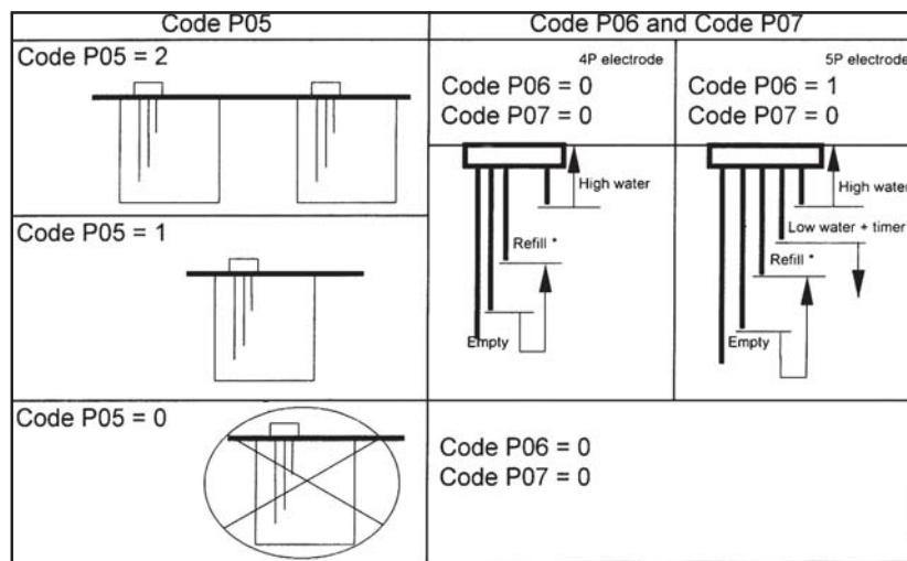
Note 1. \* Short circuit E12-E15, E22-E25 (when using the dual tank system) with the jumper cable (included).
