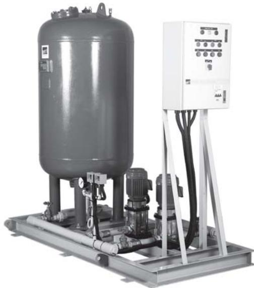
**EBARA Hydro-pneumatic booster system uses EBARA stainless steel pumps with one or more pressure tanks mounted on a common baseplate skid consisting of valves and manifolds. Custom designed electrical control panel is utilised and built to highest standard, interconnected with pump motor and control devices to ensure automatic trouble-free booster operation.**
