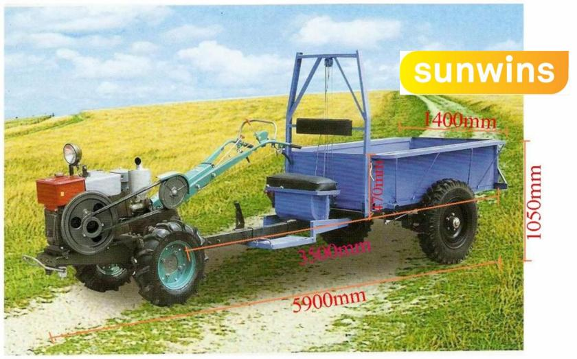
overall dimensions:5900mm x 1400mm x 470mm(Including power tiller)
